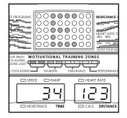
the + button (this is the button that also selects resistance level 10). While an E or an M appears in the matrix, the left display will show the total numbers of hours that the elliptical crosstrainer has been used, and the right display will show the total number of miles pedaled. When you are finished viewing this information, press the Start Program button again.
